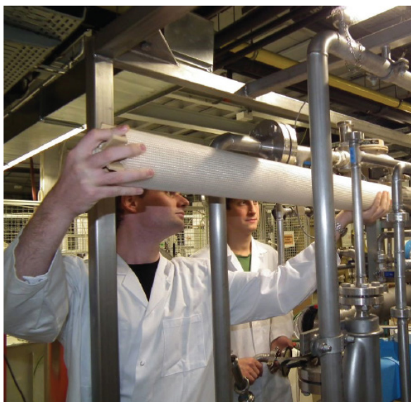
Three-stage pilot system (RO/NF/NF) with five 4“ membrane modules
