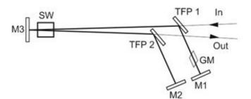
In order to trap pulses in the cavity, their polarization state is changed to PS2 for the duration of the amplification cycle. This is done by an electrooptic switch SW. The cavity is arranged so that the cavity axis intersects with itself at at least one point. The alignment of SW along the bisector of intersection angle, along with keeping the intersection angle as small as allowed by the configuration of the cavity, helps minimizing losses introduced by imperfections of the switching.
