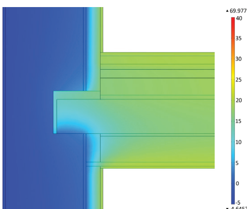
Fig 1: temp. spread w/o temp. control
