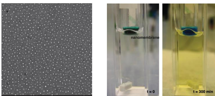
From left to right: Picture of a PHNM taken with a transmission electron microscopy; selective transport is demonstrated by separation of a mixture of methyl red with a molecular mass of 296.30 g/mol and Patent blue V with a molecular mass of 566.66 g/mol (color = green). Only methyl red passes, while Patent blue is retained. The yellow compound can be observed in the bottom.
